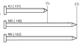
8-10 Gauge. 1½" - 2½" 4d - 8d. Full Round-Head Nails. Bright Basic and Hot Dip Galvanized Nails. Capacity 30.
